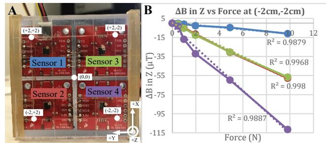
**Figure 1.** (A) Photo of custom force sensor. (B) Representative calibration data. Output from each sensor is displayed for a single force direction (Z; vertical) and position (-2 cm, -2 cm). Average  $R^2 = 0.993$ .
