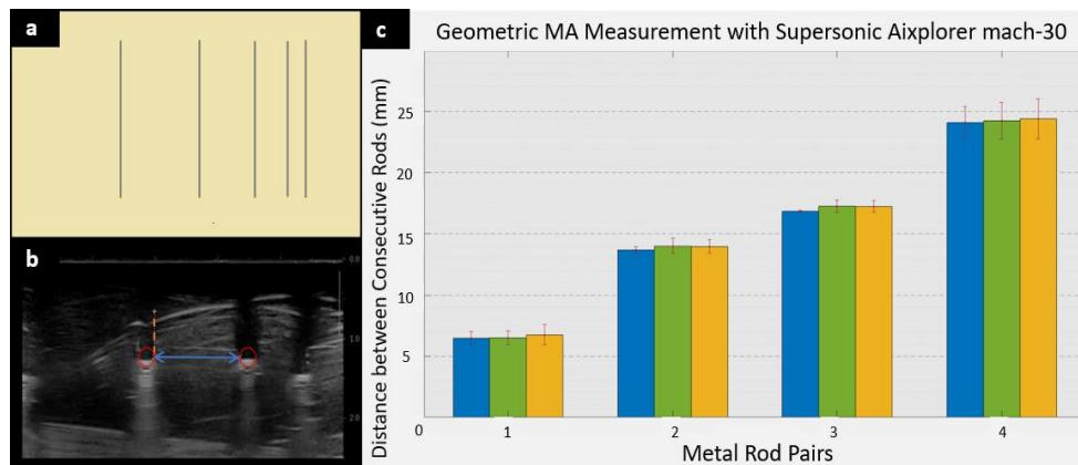
(A) Top-down illustration of the agar-phantom used, with metal rods shown in grey. (B) Transverse image of a rod pair (outlined in red) along with distance recorded between the rods (blue). (C) The data from the measurement software over the course of a week (Monday is blue, Wednesday is green, Friday is yellow).
